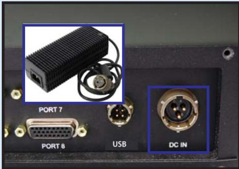
1. Locate the AC/DC power supply and AC power cable.
